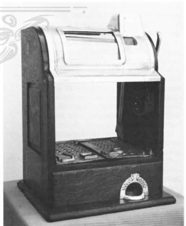
This is what the case looks like with the mechanism removed. The long slender piece is the locking bar for the rear door.
